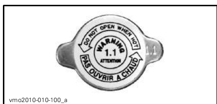
LABEL 10 - LOCATED ON RADIATOR CAP
