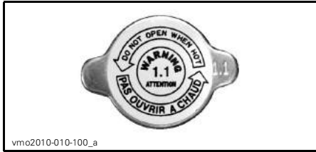
LABEL 9 - LOCATED ON RADIATOR CAP
