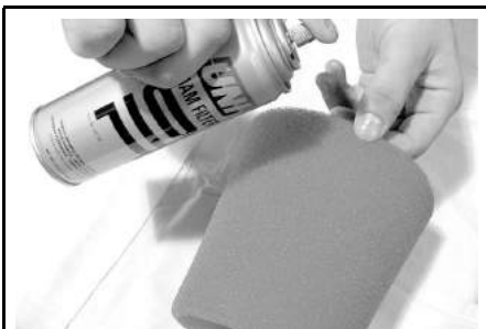
TYPICAL - OIL THE FOAM FILTER ELEMENT
