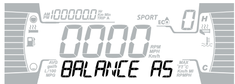
WATERCRAFT EQUIPPED WITH 4.5" DISPLAY: "SYSTEM TURN OFF : BALANCE ASSIST - HOLD CRUISE TO TURN ON"
