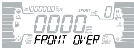
WITH 4.5" DISPLAY, THE FOLLOWING MESSAGE WILL SCROLL: "FORWARD POWER LIMITED - FRONT OVERLOADED"
