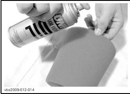
TYPICAL - OIL THE FOAM FILTER
