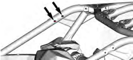
REAR OBLIQUE TUBE FASTENERS
