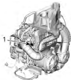
TYPICAL — ENGINE SERIAL NUMBER LABEL
