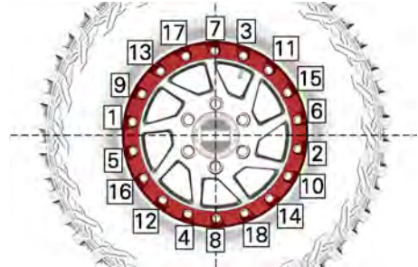
TYPICAL - TIGHTENING SEQUENCE
