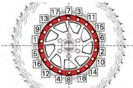
TYPICAL - TIGHTENING SEQUENCE
