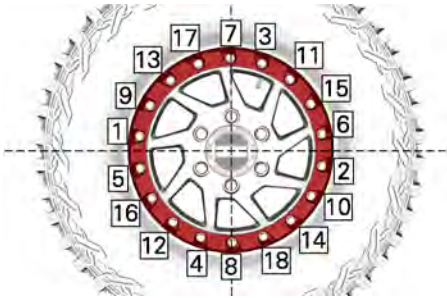
TYPICAL - TIGHTENING SEQUENCE
