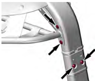
FRONT BIMINI STRUCTURE SCREWS – LH SIDE
