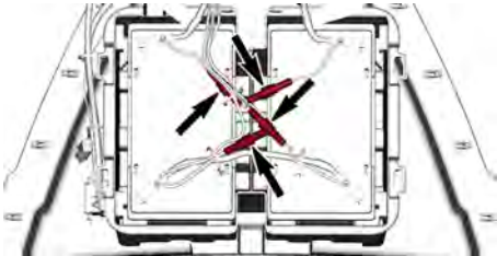
PARTS REMOVED FOR CLARITY – CHARGER FUSES
