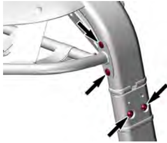
FRONT BIMINI STRUCTURE SCREWS – LH SIDE
