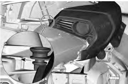
TYPICAL - ALIGNING PANELS PROPERLY
