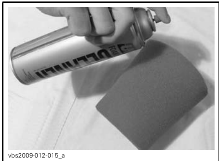
TYPICAL - SPRAY THE FOAM FILTER
