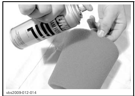
TYPICAL - OIL THE FOAM FILTER
