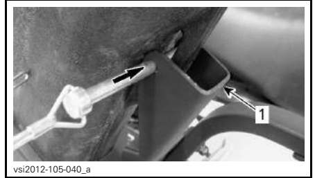
1. Bent plate of gun boot support
