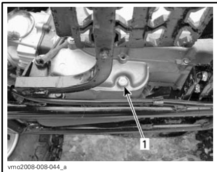
LH SIDE OF ENGINE 1. Drain plug
