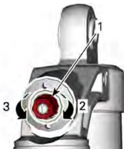
**SMORZAMENTO IN COMPRESSIONE AD ALTE VELOCITÀ (UTILIZZARE UNA CHIAVE INGLESE DA 17 MM)**
