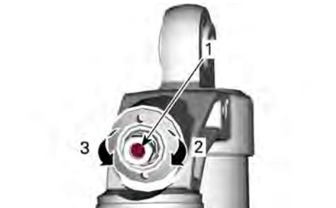
**SMORZAMENTO IN COMPRESSIONE A BASSA VELOCITÀ (UTILIZZARE UN CACCIAVITE)**
