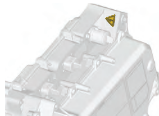
High Voltage Battery
