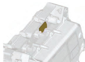
High Voltage Battery
