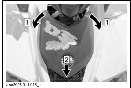
Step 1: Pull front tab from grommets Step 2: Pull cover forward then lift to remove
