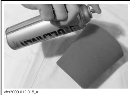
TYPICAL - SPRAY FOAM ELEMENT INSIDE AND OUT
