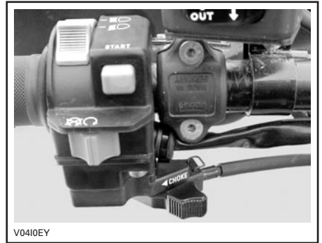
CHOKE LEVER IN THE OFF POSITION
