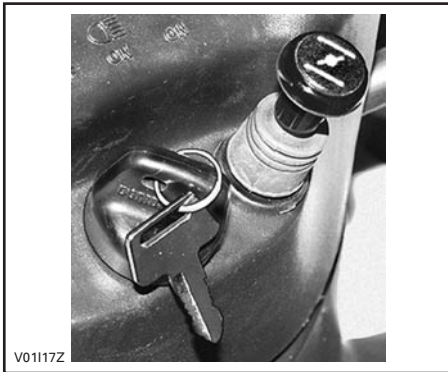
CHOKE KNOB LEVER IN THE OFF POSITION
