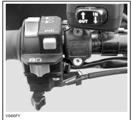
CHOKE LEVER IN THE FULL CHOKE POSITION
