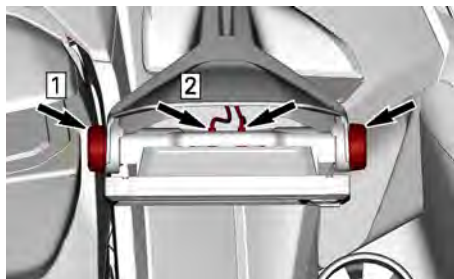
Steg 1. Lossa knopparna
