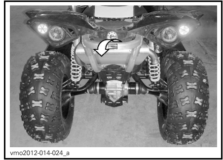
TYPICAL - REAR TIE-DOWN POINT LOCATION
