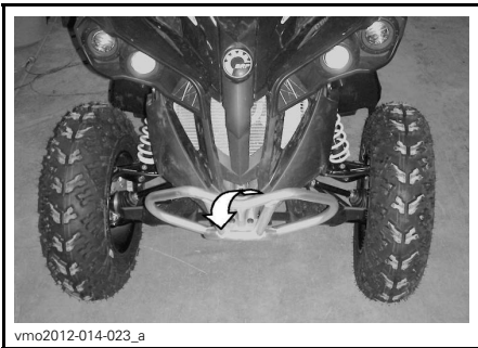
TYPICAL - FRONT TIE-DOWN POINT LOCATION
