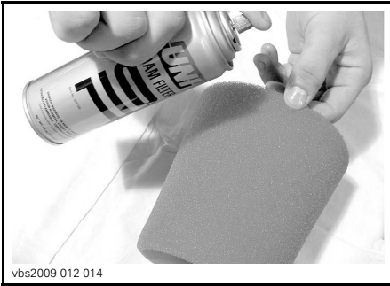
TYPICAL - OIL THE FOAM FILTER
