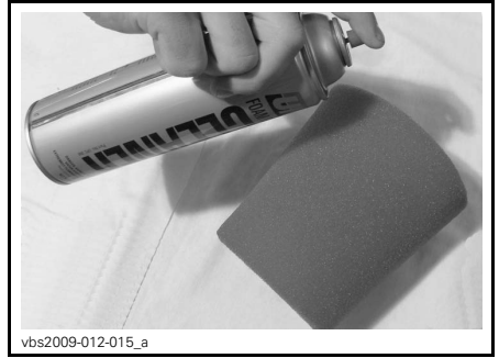
TYPICAL - SPRAY THE FOAM FILTER
