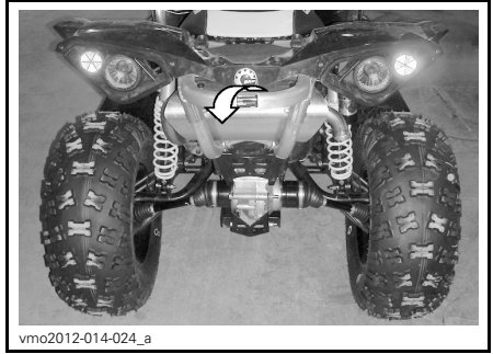
vmo2012-014-024_a TYPICAL - REAR TIE-DOWN POINT LOCATION
