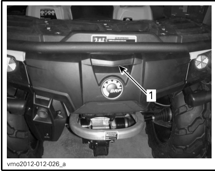
TYPICAL - 1000 MODEL SHOWN 1. Rear storage compartment latch
