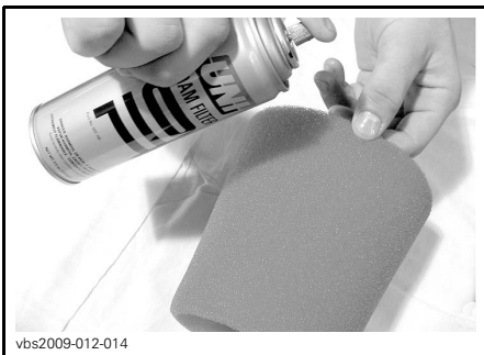
TYPICAL - OIL THE FOAM FILTER ELEMENT
