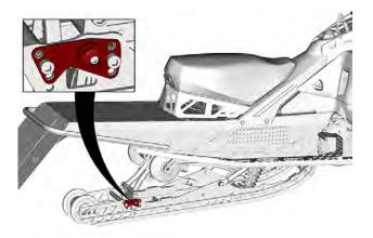
By compressing the suspension, more force is needed to initiate it's movement. This results in a faster weight transfer, which helps putting the power to the ground quicker.
