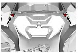
2. Lift the front of the gauge support, then slide it forward to remove it.
