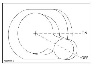
All operators of the snowmobile should familiarize themselves with the function of the emergency engine stop switch by using it several times on first outing and whenever stopping the engine thereafter. This engine stopping procedure will become a reflex and will prepare operators for emergency situations requiring its use.
