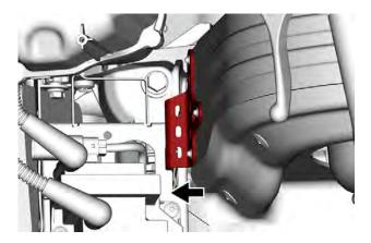
Position the rear portion of the belt guard over the retainer and secure it using the retaining pin.
