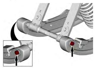
2. Rotate the axle to the desired position.
