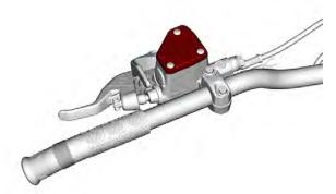
2. Remove the screws retaining the reservoir cap.
