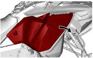
3. Slide the panel hinge off the bottom pan.
