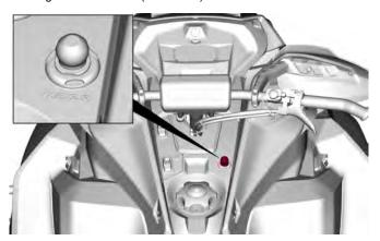
The tether cord cap must be securely snapped on the engine cut-off switch to allow vehicle operation.
