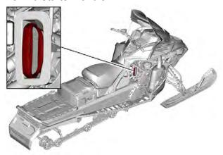
Auto-rewind type located on right hand side of snowmobile under the side panel. Open right hand side panel to access the rewind starter handle. Refer to *Removing the Side Panels* in this subsection. To engage mechanism pull handle slowly until a resistance is felt then pull vigorously. Slowly release handle.
