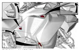
**TYPICAL** — **3 LATCHES**2. Pivot side panel around lower edge.
