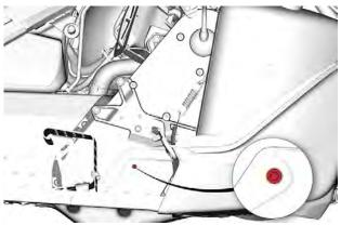
4. Remove the filler cap on top of the chaincase cover.
