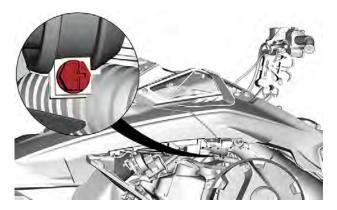
7. Remove the upper body module retaining screws on both sides.
