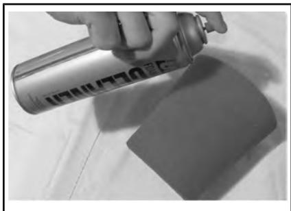
TYPISCH - SCHAUMSTOFFFILTERELEMENT BESPRÜHEN
