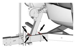
Tighten nuts to specified torque.
