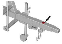
2. Removing master cylinder cap.
