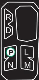
A schematic diagram of a gear shift lever. The positions are labeled: 'R' for Reverse, 'D' for Drive, 'P' for Park (highlighted in green), 'N' for Neutral, 'L' for Low, and 'M' for Manual. The lever is shown in its Park position.
