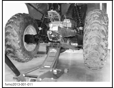
TYPICAL — BACK UP POINT LOCATION
