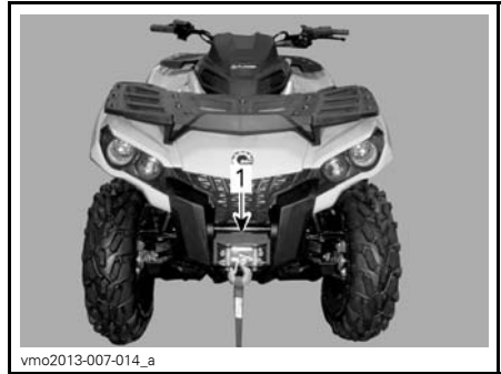
1. Front tie-down point location
