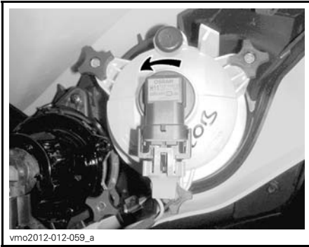
LOW BEAM ADJUSTMENT 1. Adjustment knobs
