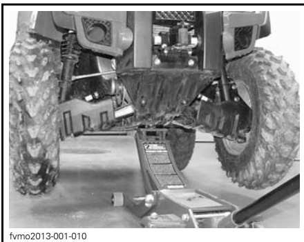
TYPICAL — FRONT UP POINT LOCATION
