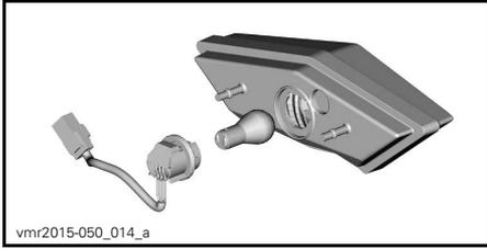
3. Remove bulb socket from taillight. Installation is the reverse of the removal procedure.
