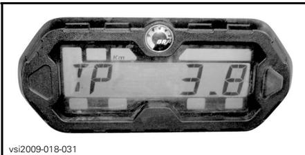
Press and HOLD the selector button for 2 seconds to reset the trip meter.
