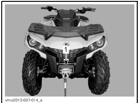
TYPICAL 1. Front tie-down point location
