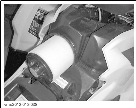
AIR FILTER REMOVAL
