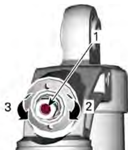
LOW-SPEED COMPRESSION DAMPING (USE A SCREWDRIVER)
