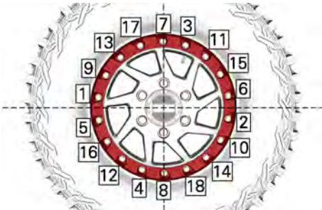
TYPICAL - TIGHTENING SEQUENCE
