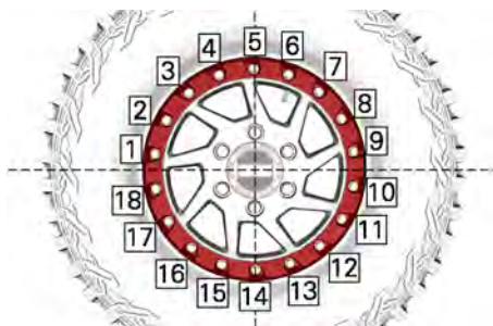
TYPICAL - FINAL TIGHTENING SEQUENCE
