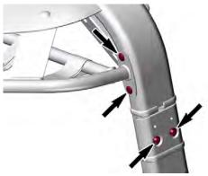
FRONT BIMINI STRUCTURE SCREWS - LH SIDE
