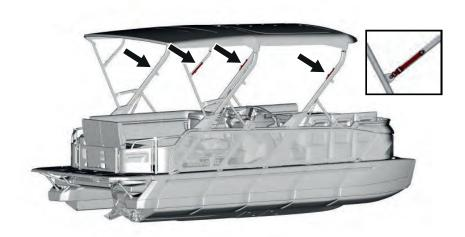
2. Unclip the rear lock on both sides by pushing down until it unclips then fold the rear structure.
