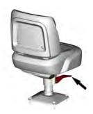
To unlock, pull up the handle and rotate the seat. To lock the seat in position, release the handle and the seat will lock in the nearest position (90 degrees increments).
