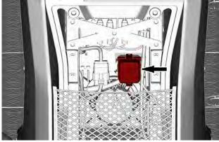
To access the engine fuse box:
