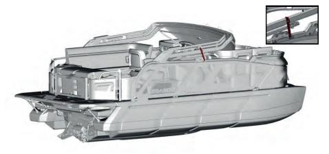
3. Raise the bimini navigation light (If Equipped). Make sure the lock is correctly engaged.
