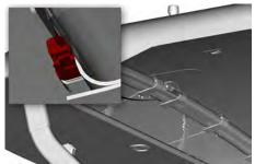
Remove the two M4 bolts and locknuts that secure the navigation to its mounting bracket. Discard the locknuts.
