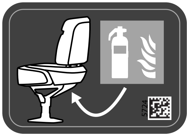
FIRE EXTINGUISHER POSITION LABEL
