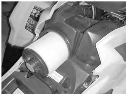
AIR FILTER REMOVAL
