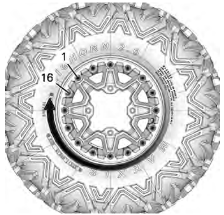
TYPICAL - FINAL TIGHTENING SEQUENCE
