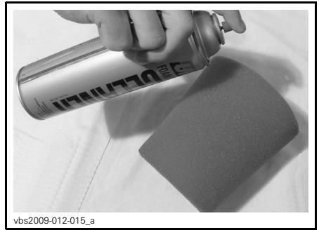
TYPICAL - SPRAY THE FOAM FILTER
