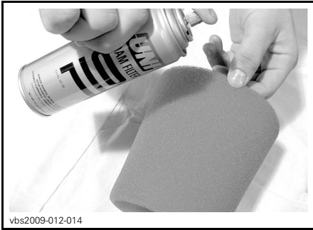
TYPICAL - OIL THE FOAM FILTER
