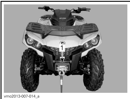
1. Front tie-down point location
