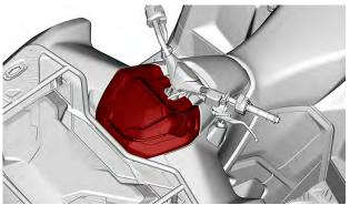
Check the coolant level, the liquid should be between MIN. and MAX. level marks of coolant reservoir.
