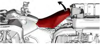
Continue lifting movement until you can release the front retaining device then completely remove seat.
