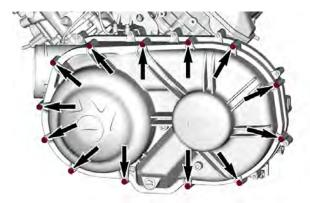
6. Remove the CVT cover and its gasket.
