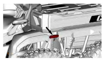
To help opening the cargo box, press down on the corner of the cargo box while moving the release handle up.
