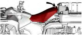
Double check that the seat is secure by giving it a tug and pulling the front to confirm proper latching.
