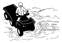
Wet brakes will affect the braking ability of your vehicle. Make sure you dry the brakes by applying them several times after the vehicle leaves the water, mud or snow. Allow greater distance for braking.
