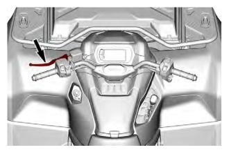
The brake lever function is to slow down or stop the vehicle.
