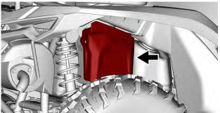
Secure battery cover with the previously removed plastic rivets.
