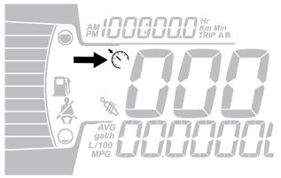
The operator can then increase the value by pressing the OFF/AC-CEL button (short press).
