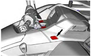
3. Unclip both locking tabs on sides of steering.
