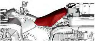
When seat rests in its position, firmly push seat down to latch. A distinctive snap will be felt.
