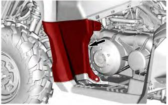
4. Disconnect the inlet air cooling duct from the CVT cover.
