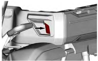
4. While holding the front handle, move the wall rearwards until the front retaining hook is visible.
