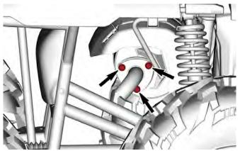
2. Remove the exhaust outlet pipe and discard the gasket.
