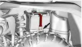
3. Connect the RED (+) battery cable first then the BLACK (-) battery cable.
