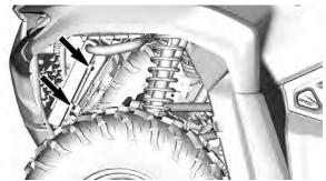
2. Disconnect the radiator fan connector.
