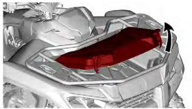
Rotate the lever located inside the storage compartment to lock the cover in the open position.
