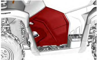
2. Remove the LH front inner fender.
