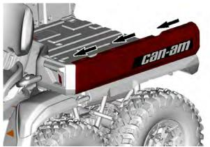
3. Lock the side wall in place by lowering the rear lock.
