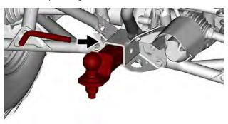
3. Secure the pin by folding the lock.
