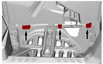
2. Secure the top of the side panel with the locking tabs.
