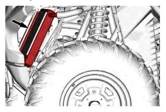
1. Remove both front air deflectors on each side of the radiator.
