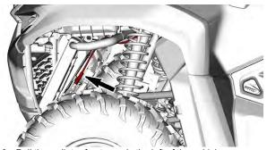
3. Pull the radiator fan towards the left of the vehicle.6. See an authorized Can-Am Off-road dealer, repair shop or person of your own choosing to check the performance of the cooling system.
