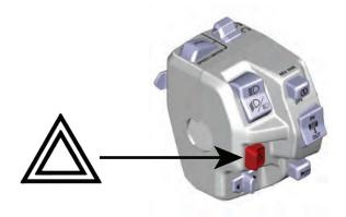
Push the button aside to activate the hazard lights. Push it on the other side to turn off.
