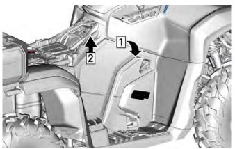
Step 1. Incline side panel Step 2. Pull upward
