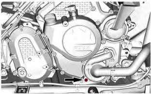
To finalize the complete emptying of the cooling system, disconnect the lower radiator hose from the water pump cover and drain the remaining coolant into a suitable container.
