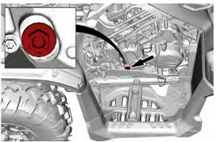
Check oil level. The oil should be level with the bottom of the oil level hole
