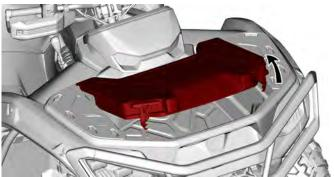
Rotate the lever located inside the storage compartment to lock the cover in the open position.
