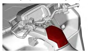
1. Push the cover button to open the compartment.
