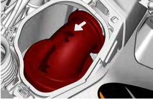
Carefully, pull the air filter adapter as well as the air filter out of the air filter housing.
