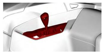
The shift lever is used to change the gearbox position.
