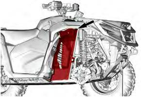
Remove the CVT intake duct.
