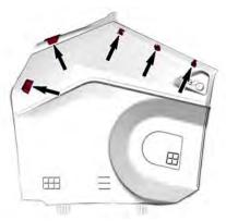
4. Incline side panel toward exterior of vehicle and pull upward to remove it from the vehicle.
