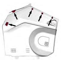
3. Lock the side panel by turning the locking latch.
