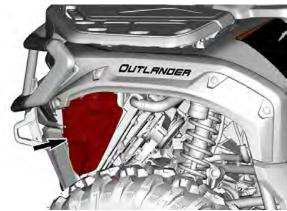
2. Disconnect the radiator fan connector.
