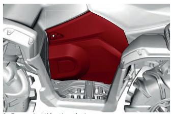
2. Remove the LH front inner fender.
