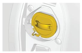
7. Ensure that the charging port connector is free of dirt, debris and water.
