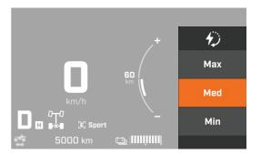
Regenerative braking is not available over 90% SOC, and is not available when the battery temperature is below 0 ° C (32 ° F). For information on how to precondition the battery to optimize performance in cold temperatures, refer to Vehicle Preconditioning, page 3-128.
