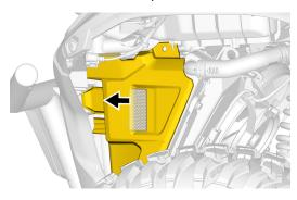
7. Install the plastic rivet to secure the front air deflectors on each side of the radiator.
