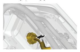
3. Connect the electrical connector to the console light. Ensure that the clip is engaged.
