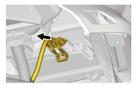
Squeeze the multifunction display connector retaining clips, then disconnect the connector.
