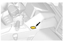
10. Secure the console with the two quarter-turn fasteners.
