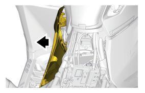
Disconnect the charging port light electrical connectors as follows:
