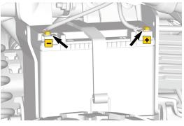
5. Connect one end of the RED jump lead to the positive (+) post of the discharged battery.
