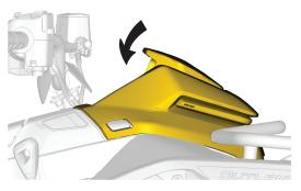
6. Push the console down to engage the locking tabs on both sides of the steering column.
