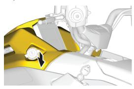
8. Press the rear-left edge of the console over the glove box tab. Make sure it clicks into place.
