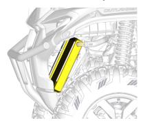
1. Remove the plastic rivet from the front air deflectors on each side of the radiator.
