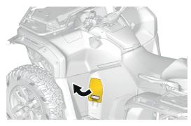
6. Remove the charging port protective cap.
