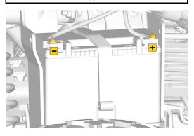
Remove the holding strap from its hook, then pull the low-voltage battery out of the frame.
