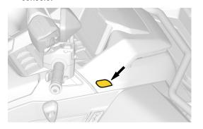
3. Lift the rear-left edge of the console to disengage the glove box tab.
