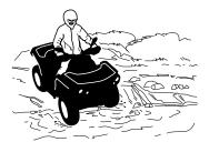
Wet brakes will affect the braking ability of your vehicle. Make sure you dry the brakes by applying them several times after the vehicle leaves the water, mud or snow. Allow greater distance for braking.
