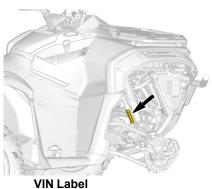
The stamped VIN is located on front member on the RH side of the vehicle.
