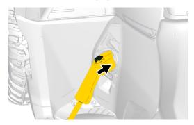
9. Ensure the EVSE charging cable is correctly locked in vehicle charging port.
