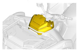
Check the coolant level. The liquid should be between MIN. and MAX. level marks of the coolant reservoir.
