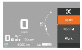
The engine mode can be changed using the **Engine Mode Selector** on the right multifunction switch. Refer to Right Multifunction Switch Operation, page 3-20.
