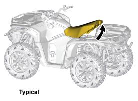
4. Continue lifting movement until you can release the front retaining device then completely remove seat.
