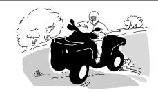
If you do get into a slide or skid, it may help to turn the handlebar in the direction of the skid until you regain control. Never jam the brakes and lock the wheels.
