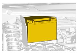
2. Secure the low-voltage battery with the holding strap.
