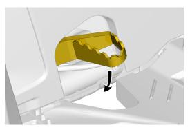
When released, the brake pedal should return to its original position.
