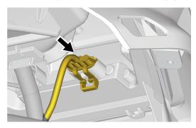
4. Push the two spade connectors onto the terminals of the 12–Volt power outlet.
