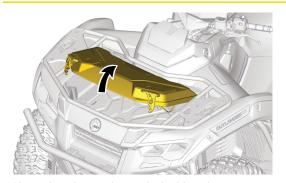
Use the lever located inside the storage compartment to lock the cover in the open position.
