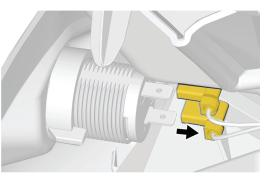
6. Unclip and disconnect the connector from the console light.
