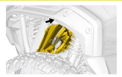
2. Connect the radiator fan connector.
