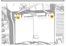
4. Tighten post screws to specification.
