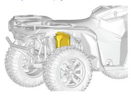
4. Remove the positive terminal cover and clean corrosion from battery posts before connecting the jumper cables.
