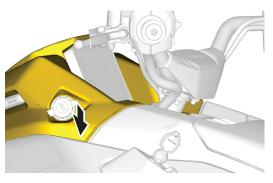
9. Ensure that the button on the right side of the console is engaged.
