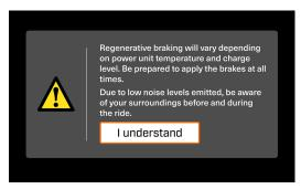
When decelerating, energy is returned automatically to the high-voltage battery. The level of returned energy and deceleration depends on the battery temperature and battery state of charge, but also on the regen mode selected. Three regen modes can be selected (Min, Med, and Max) to adjust the level of deceleration according to your preference. The MAX settings will allow more deceleration and more energy to be returned to the battery, and less brake usage.
