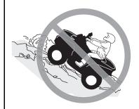
Never press the accelerator lever suddenly or make sudden gear changes. The vehicle could flip over backwards.
