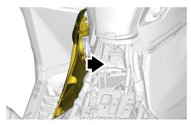
4. Install the two screws holding the side panel to the charging port support. Tighten to specification.
