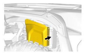
6. Secure the low-voltage battery cover with the previously removed plastic rivets.
