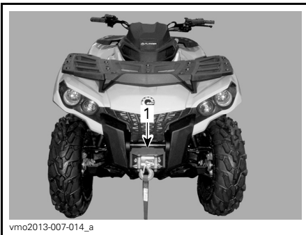
1. Front tie-down point location
