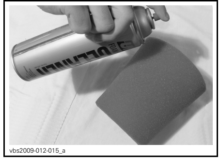
TYPICAL - SPRAY THE FOAM FILTER
