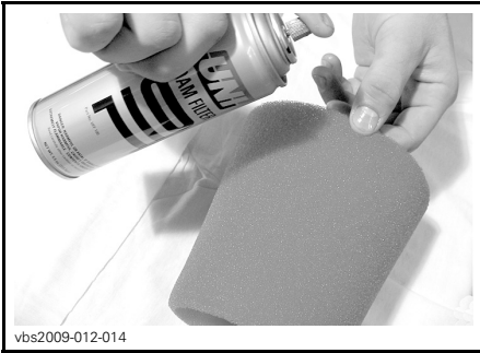
TYPICAL - OIL THE FOAM FILTER
