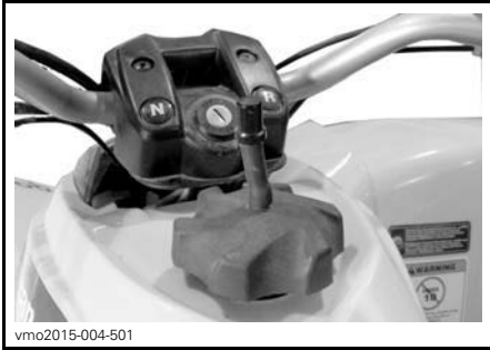
TYPICAL — FUEL TANK CAP
