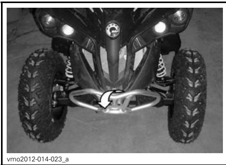
TYPICAL - FRONT TIE-DOWN POINT LOCATION
