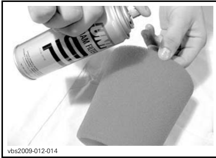
TYPICAL - OIL THE FOAM FILTER
