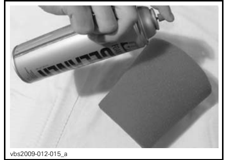
TYPICAL - SPRAY THE FOAM FILTER
