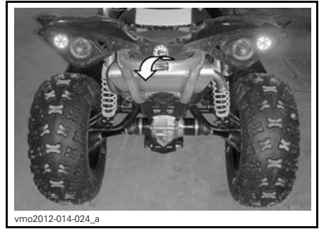
TYPICAL - REAR TIE-DOWN POINT LOCATION
