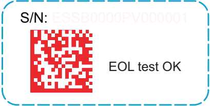
High Voltage Battery Serial Number Label
