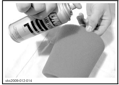
TYPICAL - OIL THE FOAM FILTER ELEMENT
