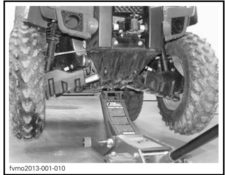
TYPICAL — FRONT UP POINT LOCATION
