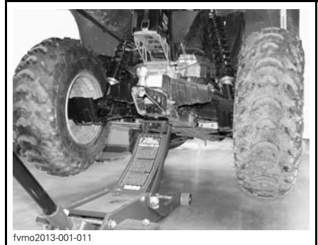
TYPICAL — BACK UP POINT LOCATION
