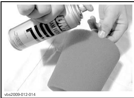
TYPICAL - OIL THE FOAM FILTER ELEMENT
