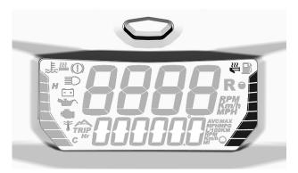
Heated grips and throttle lever will be OFF when there are no bars displayed on the gauge.
