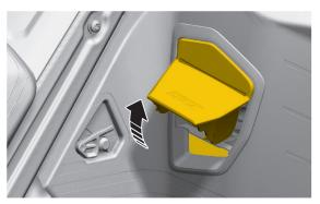
Ensure that the charger socket is free of dirt, debris and water. 6. Insert the EVSE charging cable into the vehicle charging port.
