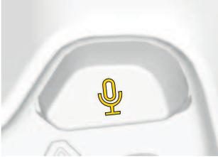
Used to trigger the voice assistant of the phone. The operator must have a phone and a headset connected via Bluetooth to use this function.
