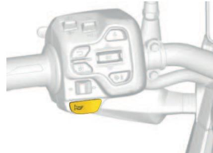
Press the button to activate the horn.
