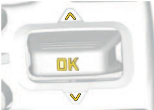
Move the button up or down to navigate through the multifunction display options.
