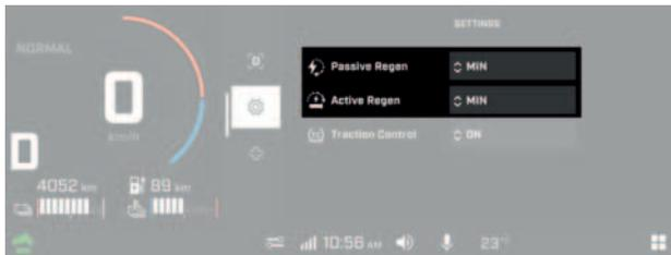
The availability of regenerative braking will vary based on these settings and other parameters such as the state of charge and temperature of the high voltage battery. The Multifunction display will always show the currently available regenerative braking capability as described in the [Multifunction Display, page 3-34](#) section.
