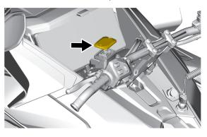
Add fluid as required. Do not overfill. Use only the recommended brake fluid. Refer to Recommended Brake Fluid in this subsection.
