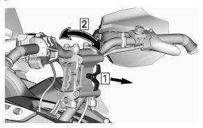
Move the handlebar back and forth to make sure the mechanism is securely engaged.
