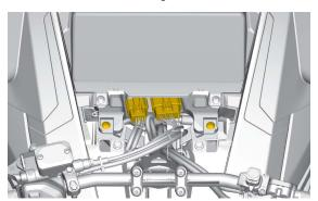
4. Remove the upper body module retaining screws on both sides.
