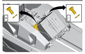
4. Remove the battery hold down bracket.
