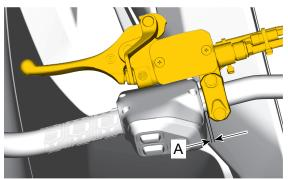
A. 0 to 5 mm (0 to 0.197 in) between the handlebar point and side of the brake lever
