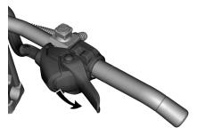
Thumb accelerator position : push downward to rotate accelerator housing
