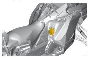
The charging connection port is located to the lower right of the driver's view. It is set up to accept both Level 1 or 2 charging. Level 1 charging uses a 120 V AC power source, while Level 2 uses a 240 V AC power source. Level 2 charging is well-suited to quicker charging situations.
