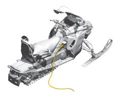
The vehicle display will switch to the charging screen. Charging will continue until the battery is fully charged or the EVSE is disconnected.
