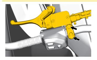
2. Locate the reference mark on the handlebar and respect the distance and rotation limits.
