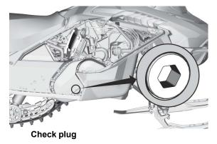
The oil level must reach the threaded hole.
