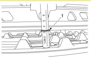
1. Deflection O-ring aligned with slider shoe
