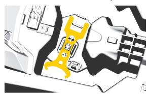
3. Slide the headlight adjustment tool short end into the hole.
