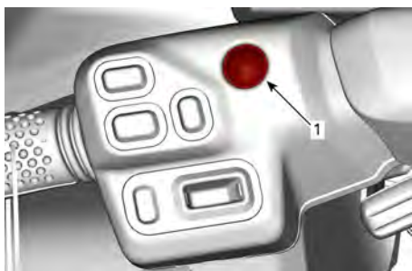
TYPBILD – MOTORNS START-/STOPP-KNAPP
