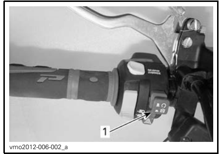
1. Emergency engine stop switch
