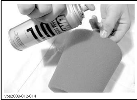
TYPICAL - OIL THE FOAM FILTER
