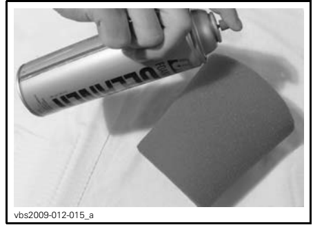
TYPICAL - SPRAY THE FOAM FILTER
