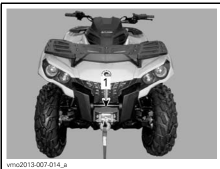
1. Front tie-down point location
