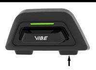
Hold the configuration button for 3 sec to access the configuration menu. You can then go to vehicle pairing by tapping the "up" button twice. Tap the center button to select "vehicle pairing". Then, on your vehicle display, go to Bluetooth settings and select your VIBE UNIVERSAL product in the list of available devices.
